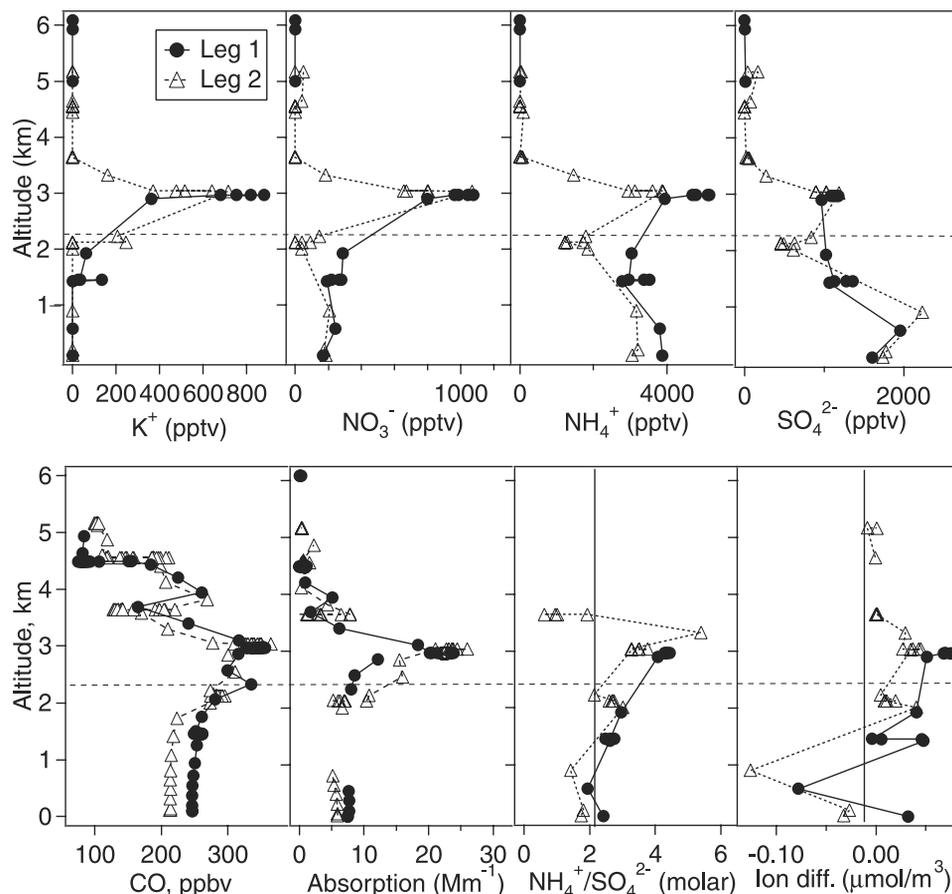
**Figure 3.** Vertical profiles for various species measured in the region of the biomass burning plume of P-3B flight 10. Closed circles are for leg 1 and open triangles are for leg 2. A temperature inversion at  $\sim 2$  km asl separates the biomass burning plume from a surface-level pollution layer.
